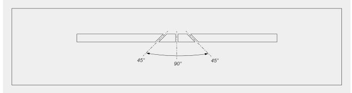
Mechanical adjustment of intermediate angles
