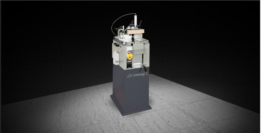
Single-head, rising blade cutting-off machine designed for cuts at 90°, 45° left and right and intermediate angles.
