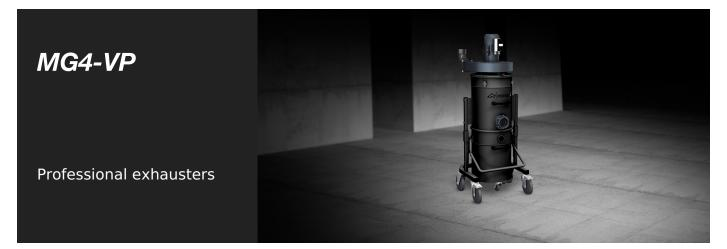
Swarf extraction system from work units with independent power supply and automatic start from machine. Ideal for aluminium and PVC. The use of a high-capacity fan, makes it suitable for various extraction requirements. A wheelmounted, quick-release, automatic vibrating filter and collection tank cleaning system, for the quick and easy disposal of exhausted material.
