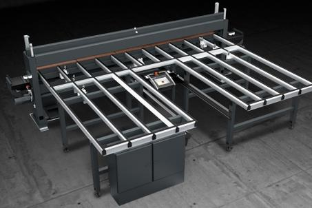
MOD-END RIFILA is a semiautomatic-cycle trimming machine for PVC frames with two controlled axes. It is equipped with a CN cutting unit with adjustable advancement speed.
