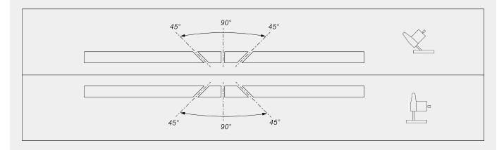
Mechanical adjustment of intermediate angles
