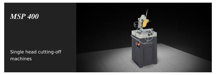
Single-head, descending blade cutting-off machine with left loading side, rotation of the cutting head to 45° (left and right) and manual tilting by 45° referred to the horizontal axis.
