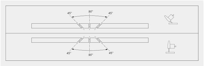
Mechanical adjustment of intermediate angles
