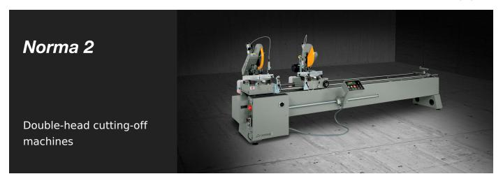
Electronic double-head cutting-off machine with automatic movement of the mobile head. Manual rotation (45° left and right) and tilting (45° in relation to the horizontal axis) of the cutting units. 400 mm-blade Available with a useful cut of 4 m or 5 m in length.
