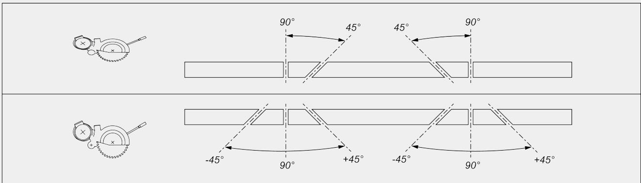
Mechanical adjustment of intermediate angles
