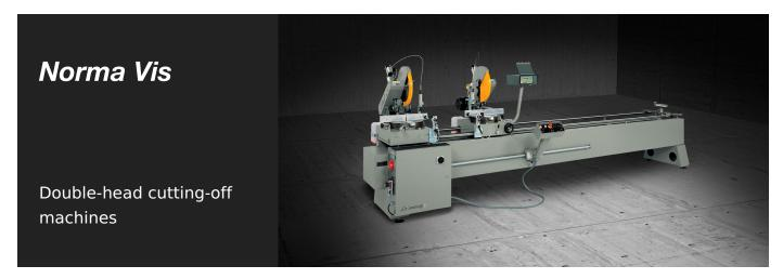
Double-head cutting-off machine with manual movement of the mobile head with digital quota visualizer (Norma Vis). Manual rotation (45° left and right) and tilting (45° in relation to the horizontal axis) of the cutting units. 400 mmblade Available with a useful cut of 4 m or 5 m in length.
