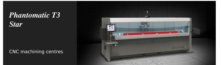
Machining centre CNC with 4 controlled axes, used for working bars of aluminium, PVC, light alloys in general and steel pieces up to 3 mm. It has a 4 tool magazine, with the possibility of hosting 2 angular units and one milling disc. The presence of the rotary work table (CN axis) allows machining at any angle from - 90° to + 90° and on the two heads with a double output angle machining head, with the table at 0°. All CNC axes are absolute and do not require resetting upon machine restart.
