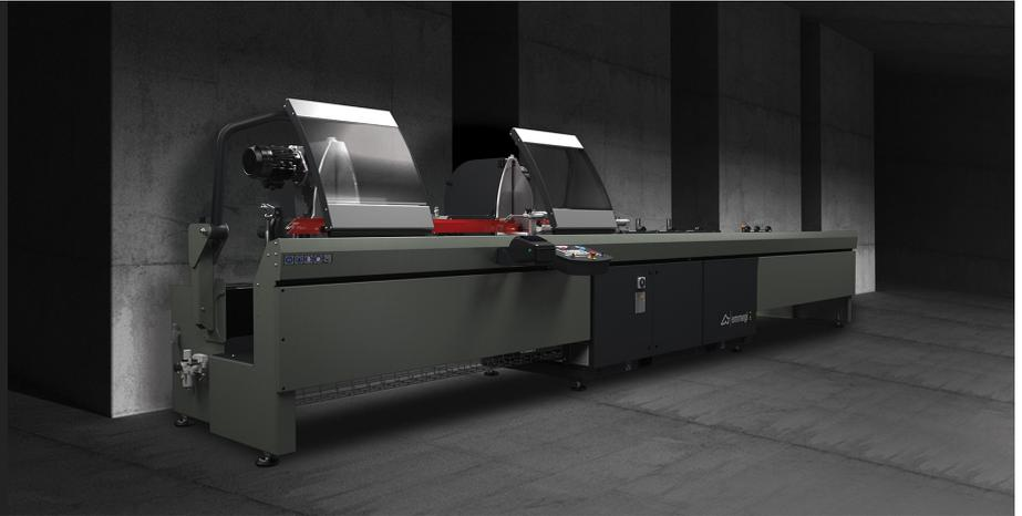
Electronic twin-head cutting-off machine with frontal blade Electronic twin-head cutting-off machine with the moving cutting head powered by brushless motor with numerical control system. Pneumatic control of the angular setting from 90° to 22°30' (external) with mechanic adjustment of intermediate angles. Hydropneumatic blade feed. Available in two versions with 4000 and 5000 mm cutting length.
