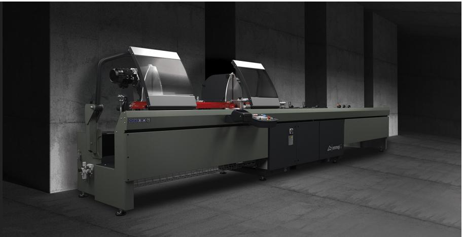
Electronic twin-head cutting-off machine with frontal blade Electronic twin-head cutting-off machine with the moving cutting head powered by brushless motor with numerical control system. Pneumatic control of the angular setting from 90° to 22°30' (external) with mechanic adjustment of intermediate angles. Hydropneumatic blade feed. Available in two versions with 4000 and 5000 mm cutting length.
