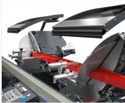
**Virtual axis for cutting units inclination**
