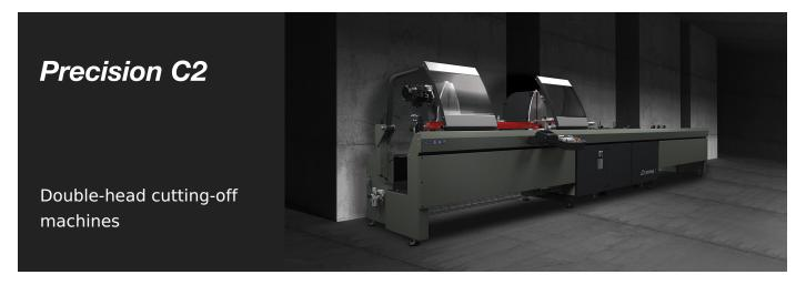
Electronic twin-head cutting-off machine with frontal blade Electronic twin-head cutting-off machine with the moving cutting head powered by brushless motor with numerical control system. Pneumatic control of the angular setting from 90° to 22°30′ (external) with mechanic adjustment of intermediate angles. Hydropneumatic blade feed. Available in two versions with 4000 and 5000 mm cutting length.
