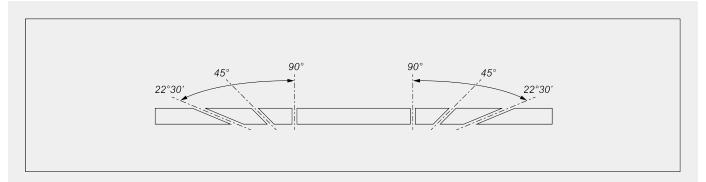
Mechanical adjustment of intermediate angles
