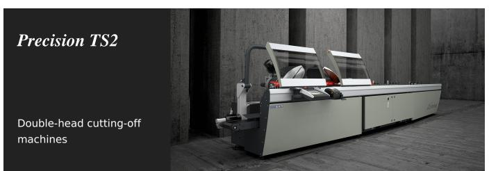
Twin-head cutting-off machine with 3 controlled axes, automatic traverse of the moving cutting head and electronic control of every angular setting from 45° (internal) to 15° (external) with accuracy of 280 places on each degree. The blade feed is controled by two hydro-pneumatic cylinders.
