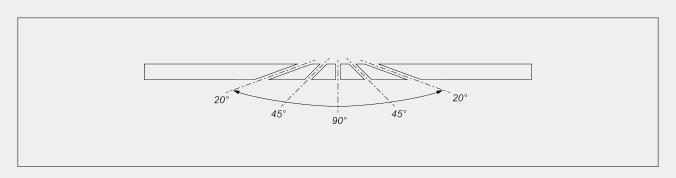
Mechanical adjustment of intermediate angles
