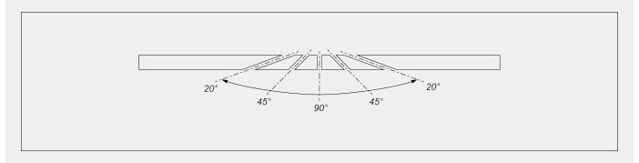
Mechanical adjustment of intermediate angles
