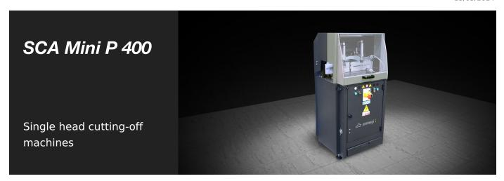
The single head rising blade cutting-off machine, with left loading side, for cutting at angular settings from 15° to the left to 15° to the right and intermediate angles. Available with pneumatic blade feed.
