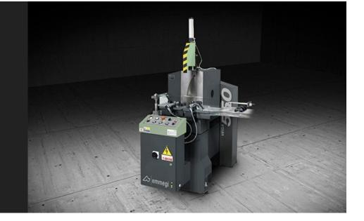
Single-head cutting-off machine with horizontal blade feed and left loading side, pneumatic double side tilting of the cutting head in fixed positions: 45° to the left, 90°, 45° and 22°30' to the right. A special positive stop also allows cutting at intermediate angles.
